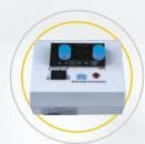
The **VERIFY Biological Indicator Incubator** has a set point of 57 °C for use with VERIFY V24 Self-Contained VH202 Biological Indicators.
