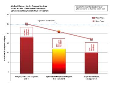
**Excellent Spray Arm Movement:** No difference in motion from water alone; arm rotation at optimum speed creating high impingement and full cascade on loading doors
